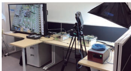
Demonstration of 4K uncompressed video transmission using GI-POF
