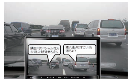
Figure 1: Information exchange by visible light communication between LED break lamps
