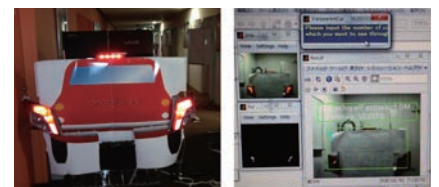
Figure 2: A prototype of visual light communication between LED break lamps
